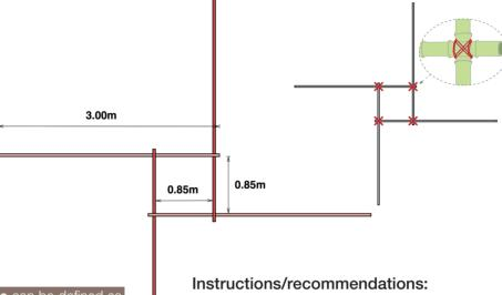
**Note:** The **reciprocal frame** can be defined as a structure made up of mutually supporting poles placed in a closed circuit. In this shelter 4 poles are overlapped in turn to create a **self-supporting** reciprocal frame roof.
